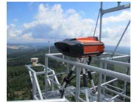
Fig.2: WIND IRIS, turbine mounted pulsed multi range LiDAR installed on turbine roof
